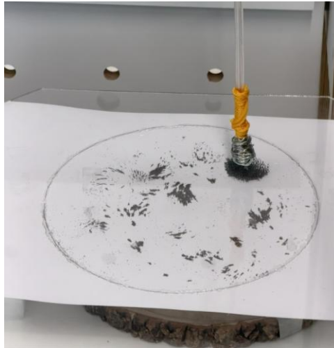
Figure 11. Early prototype with iron filings, showing how magnetic interaction could leave visible traces on the plate. Source: authors.
