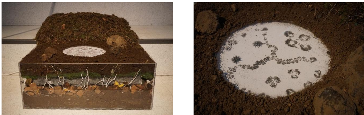
Figure 14. Final soil box with the magnetic plate integrated into the layered underground structure. Source: authors.
