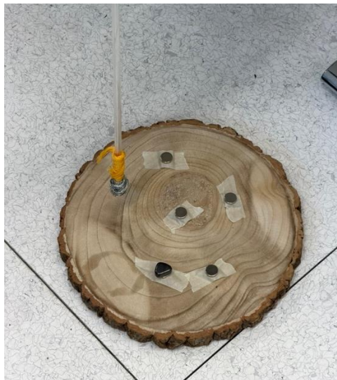
Figure 10. First prototype of the magnetic pendulum, used to test how different magnet arrangements influenced the pendulum's motion. Source: authors.
